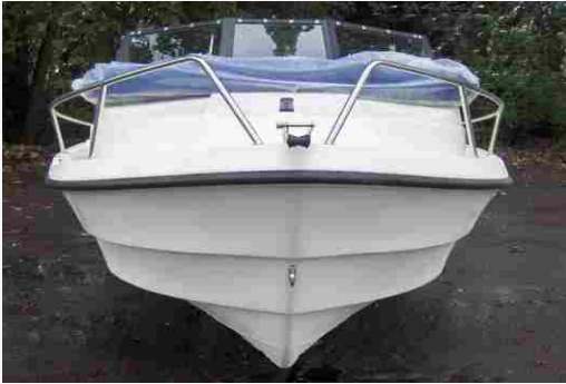
From this angle you notice the wide chine and above that is a feature line that acts as a deflector.
