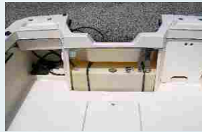
27 Gal. Gas Tank & Battery Storage
