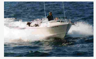
Notice how the water and splash is deflected away from the boat by the chine and feature line.
