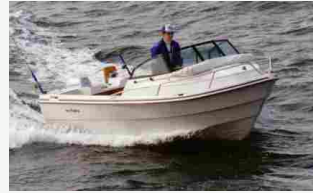
Notice how the water and splash is deflected away from the boat by the chine and feature line.
